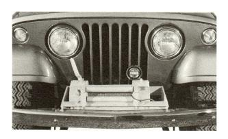
Combining strong, light-weight housing and long-wearing gears with seamless steel cable drum and high-strength shafts, mechanical front-mounted winches are available for vehicles equipped with the Dauntless V-6 engine. (See Section 25 of your 'Jeep' dealer's Special Equipment Manual.)
