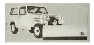
Available for all models, snow plow has 78-inch blade width and features a replaceable 6-inch high cutting edge, safety spring trip and self-locking shear pin. Blade can be quickly removed to permit conventional use of vehicle and re-installed without special tools. Choose from hydro-electric and full hydraulic lifts . . . power angling and V-blade also available. (See Section 20 of your 'Jeep' dealer's Special Equipment Manual.)
