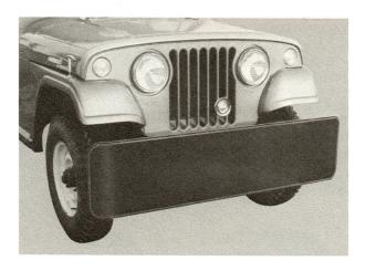
Formed of a %-inch thick steel plate, push plate design also allows vehicles to be pushed around corners. Also available with cutout for approved winch or snow plow attachments. (See Section 5 of your 'Jeep' dealer's Special Equipment Manual.)
