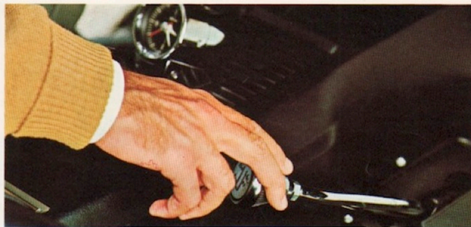
Direct linkage to the transfer case makes it an easy shift from 2wd to 4wd and back again.
