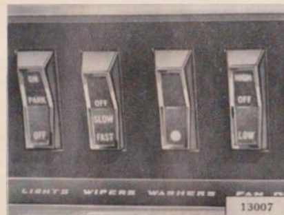
FIG. 11—WINDSHIELD WIPER AND WASHER CONTROLS
