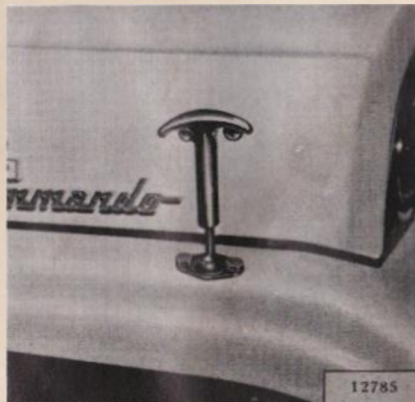
FIG. 16—HOOD RELEASE LATCH
